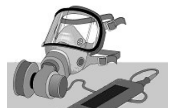
Air purifying full facepiece respirator equipped with P100 cartridges.
