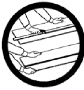
Cutting asbestos-containing wall board by hand.
