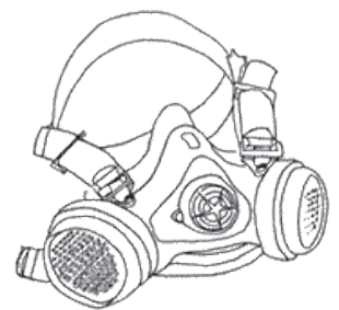
Air purifying half-mask respirator equipped with P100 cartridges.
