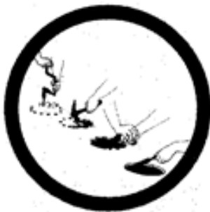
Use of hand tools to remove wall boarding containing asbestos.
