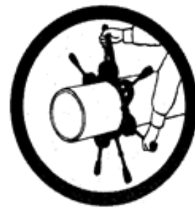
Cutting asbestos-containing pipe by hand.
